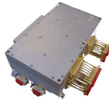
FEEU : 2 low noise Electronics units
