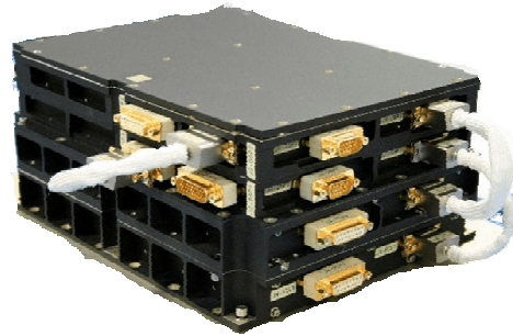
ICU : digital control laws, data conditioning
