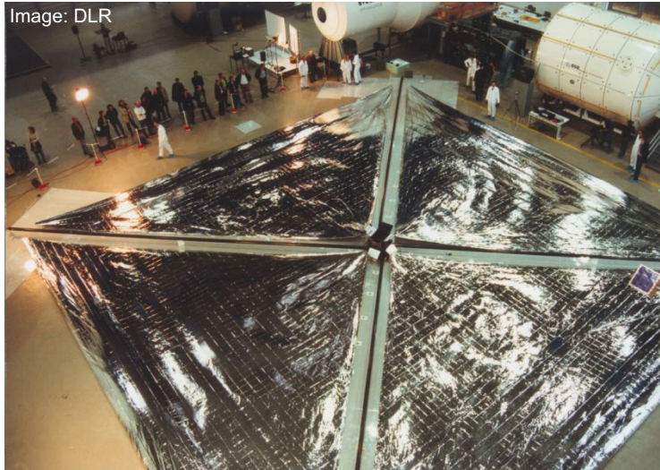
DLR / ESA: Ground deployment experiment for a 20 m x 20 m, 35 kg solar sail at EAC, Cologne, Germany (December 1999)
