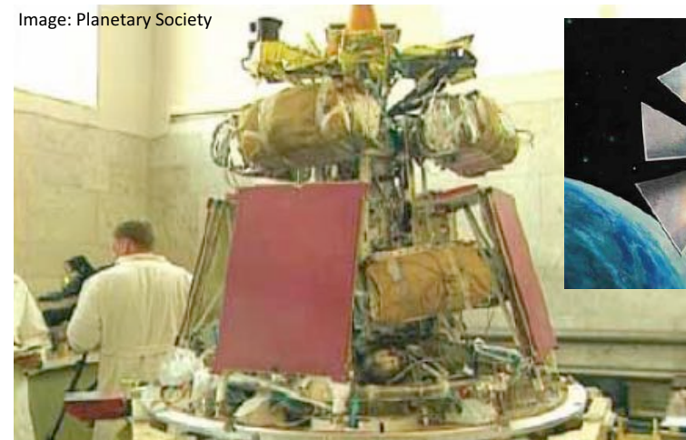
Planetary Society: Cosmos 1, 30 m „flower“, 105 kg, planned orbital altitude: 1000 km, launcher failure (June 2005)
