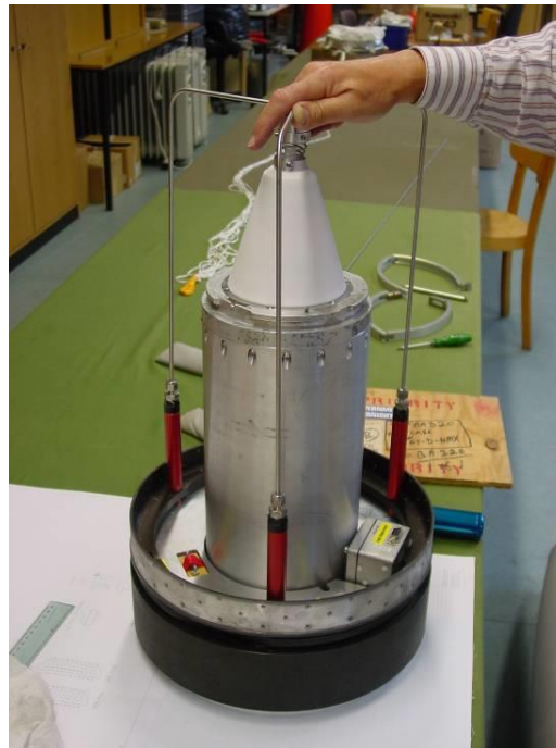
Figure 5-2: REXUS Nose Cone Experiment (Underneath Ejectable Nose Cone)
