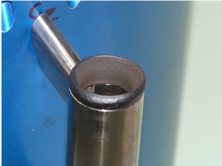
Figure 50. Insulation ring melted during the flight
