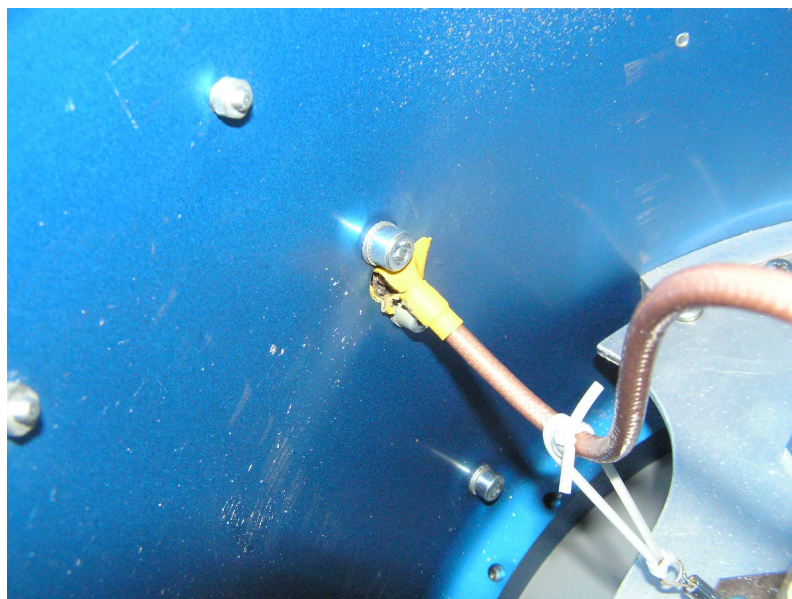
Figure 49. The attachment of the triaxial cables are damaged
