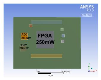
Picture 7 Power dissipation on the baseboard
