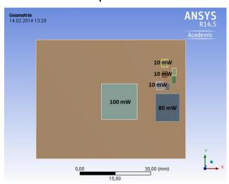
Picture 8 Power dissipation on the ARM Computer Board
