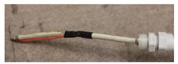
Picture 14: Broken antenna after the flight.
