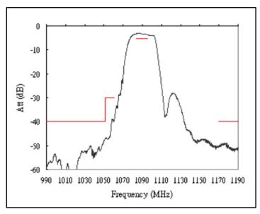
Figure 4 TA0232A transfer function
