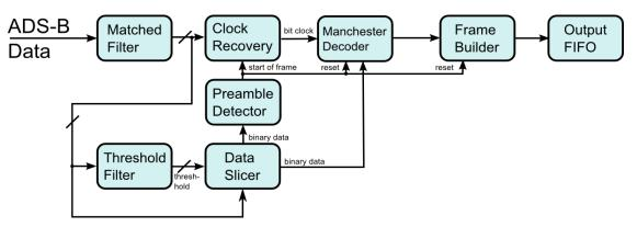
Figure 6 Signal processing concept
