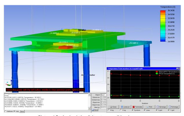
Picture 4 Static simulation (laboratory conditions)
