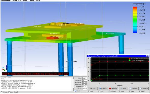
Picture 6 Static Simulation Result of -60°C environment, near vacuum
