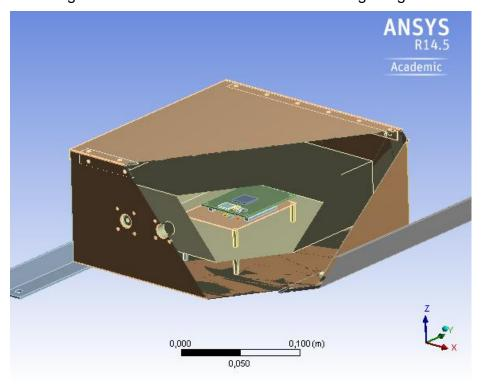
Picture 2 PCB mounting in the experiment case
