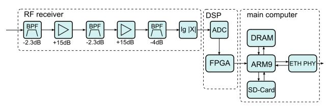
Figure 3 The electronics concept
