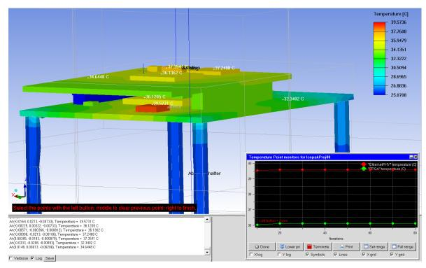
Picture 5 Temperature profile of simulated vacuum test
