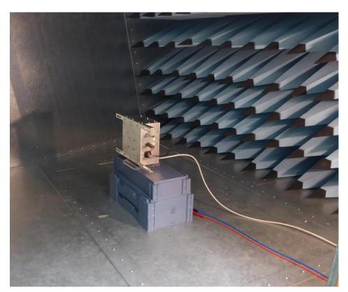
Picture 12: Experiment placed into the GTEM chamber
