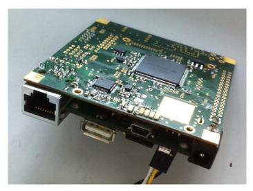
Picture 6 The built ARCA baseboard (top) and some connectors
