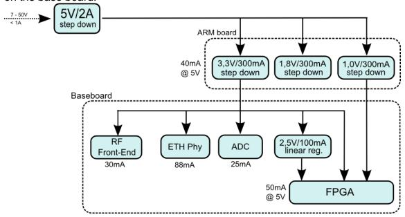
Figure 5 Power supply concept
