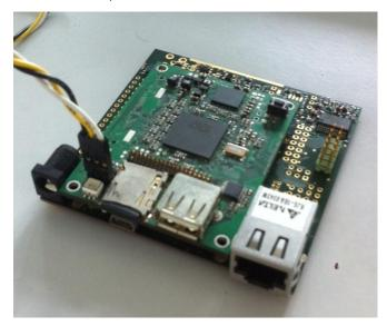
Picture 5 The built ARCA baseboard (bottom) with ARM-board (top)
