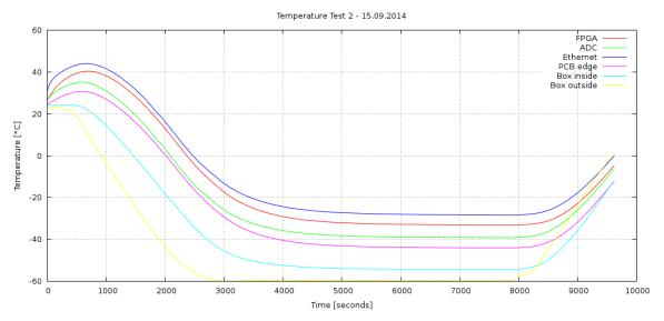
Picture 11: Temperature plot during the temperature chamber test.
