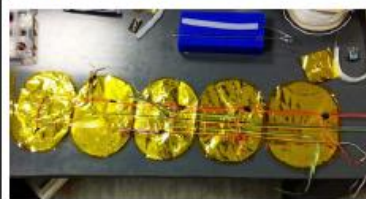
TM of one row of inflatable cells (Actuator elements can also be seen in photo)
