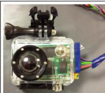
Hack-HD Camera inside housing
