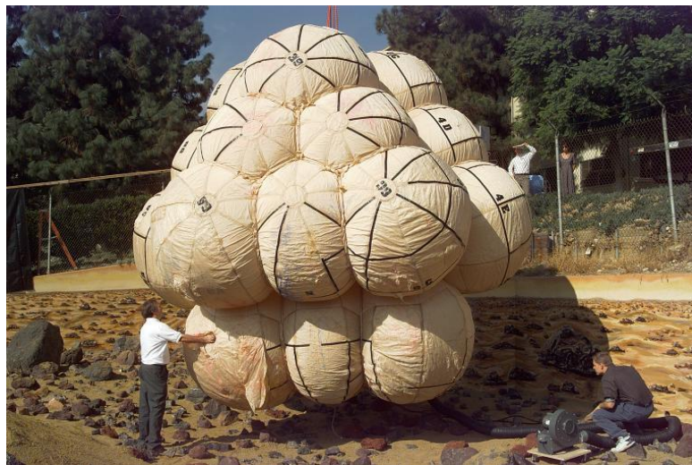
Figure 1-2: Deployment test of inflatable airbags of Mars Pathfinder mission in 1996 (source NASA)
