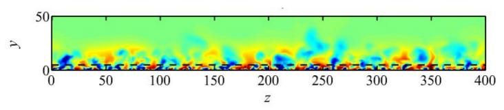
Cross-stream cut of isolevels of streamwise velocity fluctuations in an Asymptotic Suction Boundary layer flow at the verge of relaminarisation, spectral numerical simulation (Re=260), from Khapko, Schlatter, Duguet & Henningson, JFM 795 (2016).
