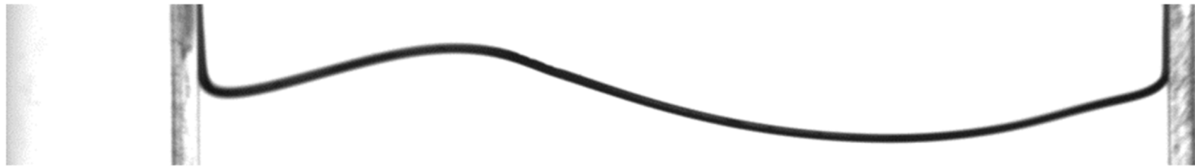
Figure 1 - Air/ethanol interface during a sloshing experiment in a Hele-Shaw cell of width 10 cm.
