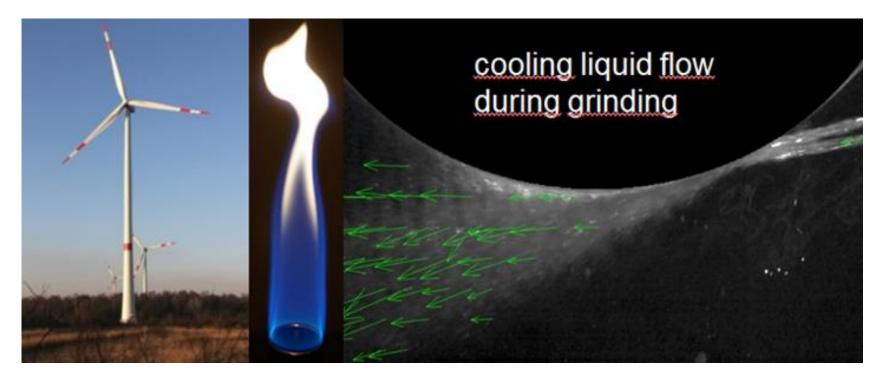
Topical in-process flow measurement tasks: Flow visualization for wind turbine engineering, combustion flow analysis and understanding the cooling mechanism during grinding
