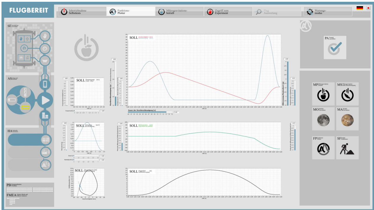
Figure 2.10: Excerpt of the intuitive Graphical User Interface (GUI) of GraviTower's Software Control Interface - view of the actual tab with the adjustable kinematics by means of the acceleration and deceleration plotter.
