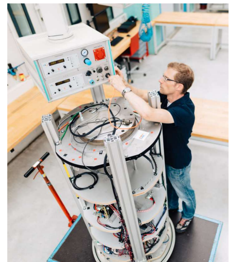
Figure 2.6: EGSE-to-capsule interface unit.
