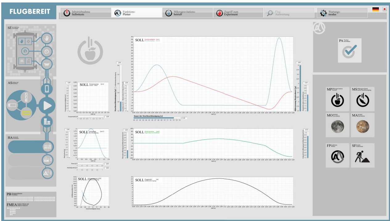
Figure J: Excerpt of the intuitive Graphical User Interface (GUI) of GraviTower's Software Control Interface - view of the actual tab with the adjustable kinematics by means of the acceleration and deceleration plotter.
