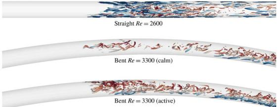
Turbulent fronts at different Reynolds numbers and geometries from [3]
