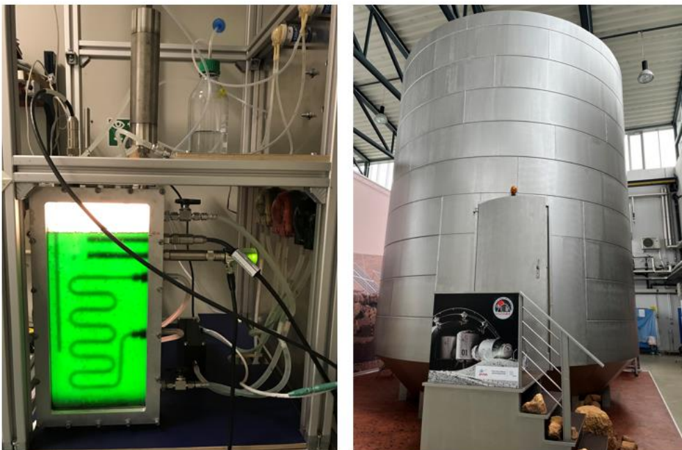
Abbildung 1 The photobioreactor as part of a bioregenerative life support system (left) and the MaMBA habitat at ZARM (right).
