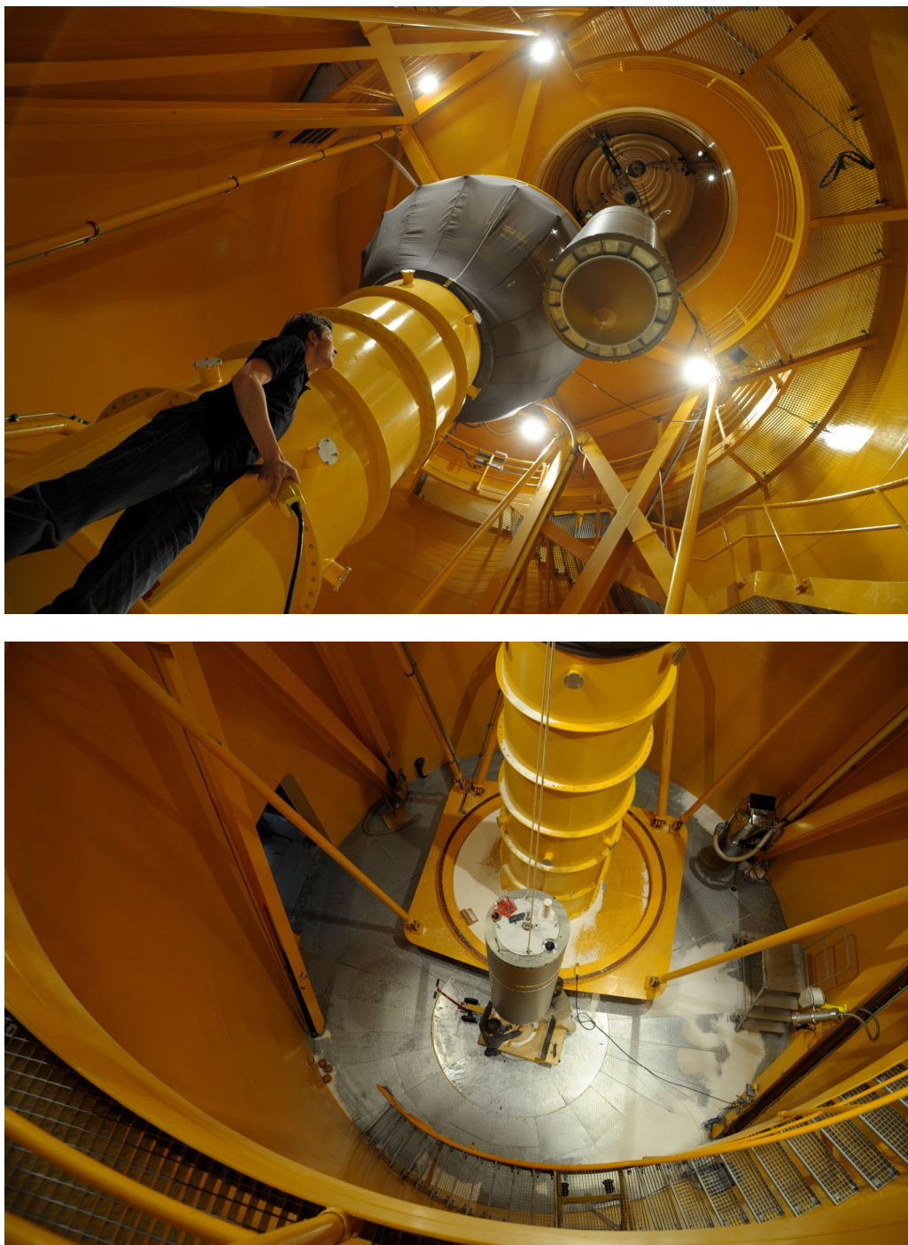
Figure 2.2: Bottom-up [top] and top-down view [bottom] from inside of the deceleration chamber - with deceleration container, drop tube, and experiment capsule during drop preparation.
