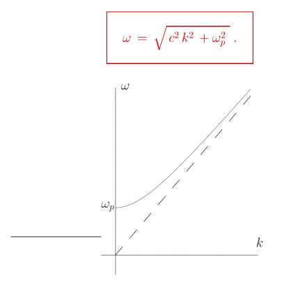
Note that the electron density  $n_e^0$  and, thus, the plasma frequency  $\omega_p$  is, in general, a function of r and t.
