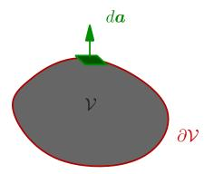
closed surface is zero, i.e., that the magnetic field has no sources. (A modification of the first Maxwell equation has been suggested where the right-hand side of (MI) is not zero. This would correspond to the existence of "magnetic sources", called *magnetic monopoles*. However, up to now there is no experimental indication that they exist.)
