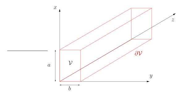
To solve the Helmholtz equation (HE) with the boundary condition (BC) for this case, we make a separation ansatz
