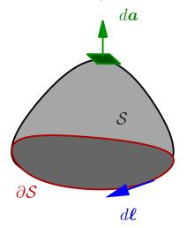
the vectorial length element along  $\partial S$ . The usual sign conventions are: If the thumb of your right hand points in the direction of da, the remaining four fingers point in the direction of  $d\ell$ . – This equation says that the temporal change of the flow of **B** through a non-closed surface equals, up to sign, the circulation of **E** in the boundary of this surface ("Faraday's law").
