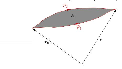
such that the boundary  $\partial S$  consists of  $\mathcal{P}_1$  with positive orientation and  $\mathcal{P}_2$  with negative orientation. Then, by Stokes theorem,
