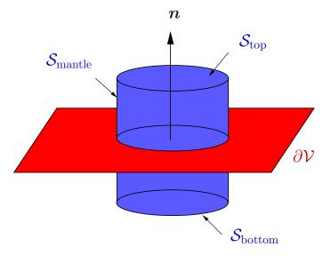
$$\int_{\mathcal{S}_{\text{bottom}}} \boldsymbol{B} \cdot d\boldsymbol{a} + \int_{\mathcal{S}_{\text{top}}} \boldsymbol{B} \cdot d\boldsymbol{a} + \int_{\mathcal{S}_{\text{mantle}}} \boldsymbol{B} \cdot d\boldsymbol{a} = 0 \; .$$
