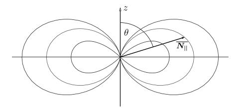
Radiation pattern of oscillating electric dipole
