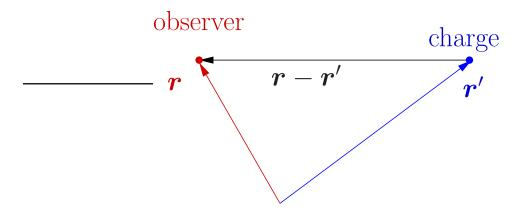
The observer at  $\boldsymbol{r}$  notices an action at time t if the charge at  $\boldsymbol{r}'$  was moved at the retarded time  $t_r = t - |\boldsymbol{r} - \boldsymbol{r}'|/v$ .
