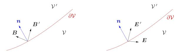
Let  $\boldsymbol{E}$  and  $\boldsymbol{B}$  be the limit values of electric and magnetic fields at a point of the boundary surface  $\partial \mathcal{V}$  if we approach it from  $\mathcal{V}$ . Similarly, let  $\boldsymbol{E}'$  and  $\boldsymbol{B}'$  be the limit values of electric and magnetic fields at a point of the boundary surface  $\partial \mathcal{V}$  if we approach it from  $\mathcal{V}'$ . Let  $\boldsymbol{n}$  be the unit vector normal to  $\partial \mathcal{V}$ .
