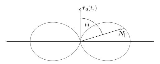
The picture shows how the "tip of the arrow"  $N_{||}$  varies if  $\Theta$  varies from zero to  $\pi$ . This is known as the "radiation pattern" of an accelerated charge.
