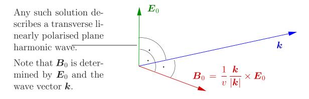
The general solution of the homogeneous wave equation is an arbitrary superposition of such waves. This can be a finite sum, an infinite series (Fourier series), or an integral (Fourier integral). A circularly polarised wave, e.g., is a superposition of just two such linearly polarised waves, see 2nd worksheet. The general form of a Fourier integral solution is given by the potentials  $V(\mathbf{r}, t) = 0$  and
