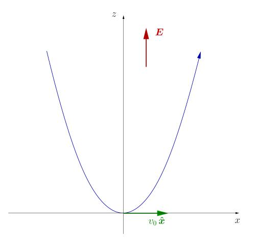
Parabolic trajecory of a charged particle in a constant electric field.
